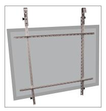
4. Hang the bracket with the mounted solar panel on the suspension. Fix the suspension with 1x screw, washer, nut M8 x 75 mm.
