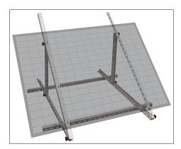
3. Attach the bracket to the surface. Use the M5 x 40 mm screws for this purpose.
