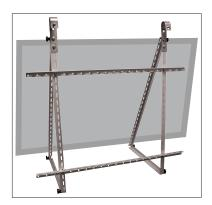
5. Hang the holder with the mounted solar panel on the suspension. Fix the suspension in each case with 1x screw, washer, nut M8 x 75 mm.
