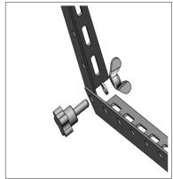
2. Mount a suspension on each of the two triangular frames as shown. Fasten the suspension with 2x screw M6 x 20mm each.
